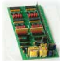
E8121BE1 Hall Interface Module PCB for LRV4
