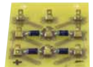
9879810 Rectifier, Full Wave Bridge, Single-Phase, 300V, 3A
