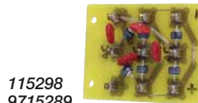
9879810 Rectifier, Full Wave Bridge, Single-Phase, 300V, 3A
