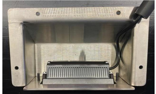
Figure 37: CabSafe 3D Sensor installed in back of transom bracket
